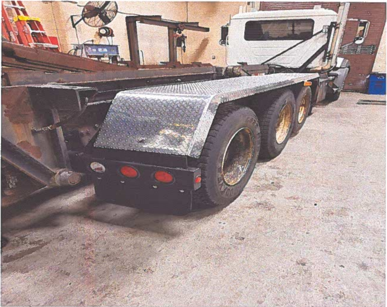
T-13 Fender repairs
