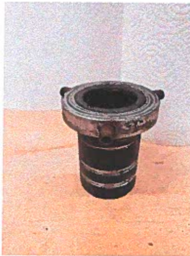
Replaced wear sleeve from RFP #1 flocculator
