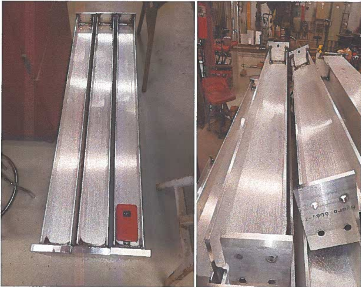
Aluminum Catwalk Components
