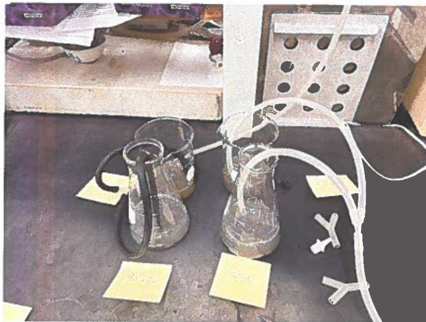
Bench Scale testing different mixtures of filtrate and bioculture ranging from 25% - 100%
