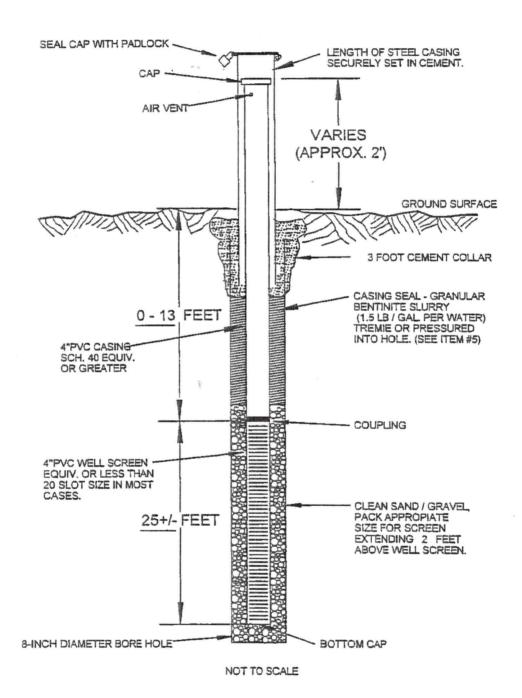
WELL Nos. 1 THRU 3, 6, 9 THRU 13, 15, 9A AND WELL No. 20
